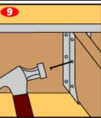
10. Where each joist crosses the beam, screw or toe-nail the joist to the beam. The deck frame is now complete. It is time to proceed with decking and railings.
